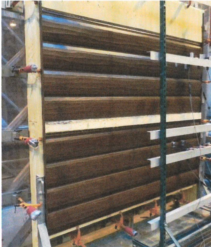
Photo No. 2 TruLog, Steel Siding, Dual Specimen Install
